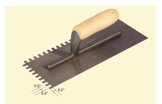
Apply bonding mortar with a 1/2 " x 1/2 " <u>NOTCHED TROWEL</u> to ensure 100% coverage.
